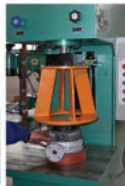
valve seat installation
